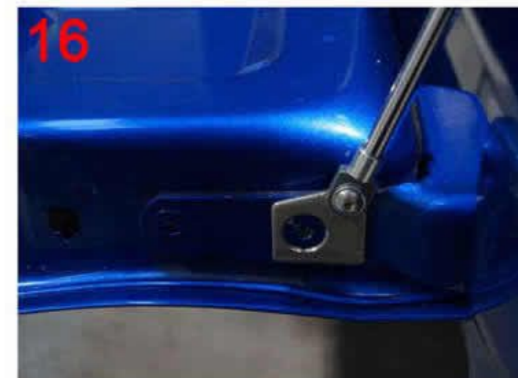
16: Install the strut as shown then replace and tighten the bolt
