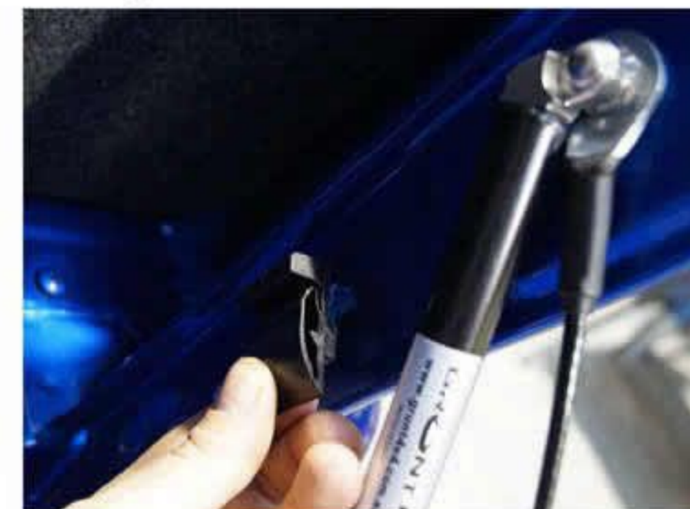
14: Remove the rubber locating blocks from the tailgate and ute tub
