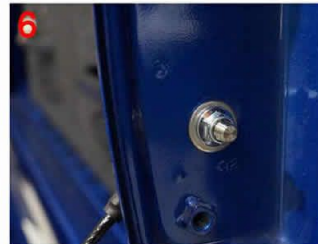
6: Place the thicker washer on the back followed by the friction nut then tighten
