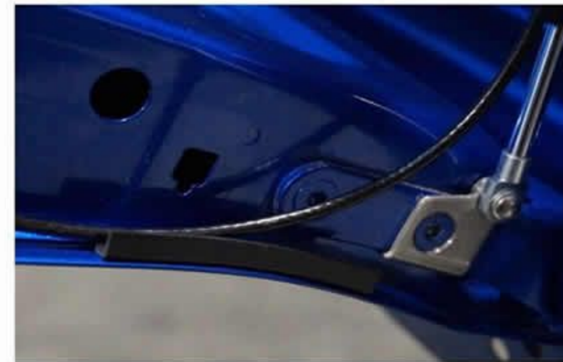
17: Install the cable locating rubber 80mm back from the body as pictured
