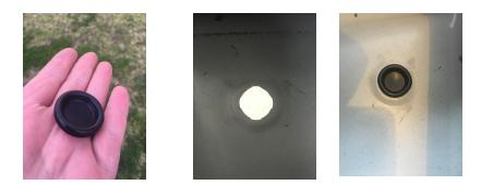
Little Black Grommet is for blocking off the rear key barrel lock. If you choose to do so. Just file out the hole a little till its round then pop the grommet in place.
