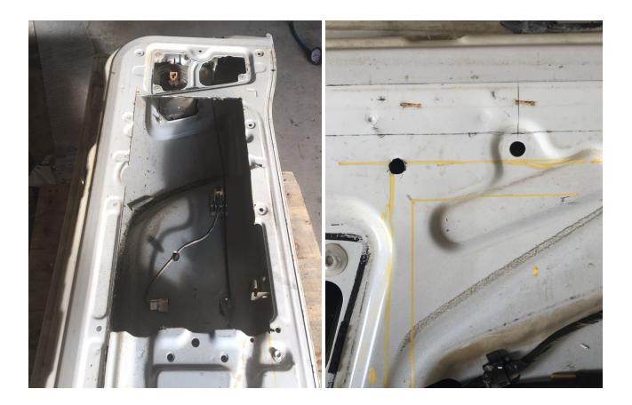
Start cutting in one corner along the line working you way around the whole tailgate, leave some small parts uncut as you go, if you cut the whole thing out in one go it will flex and vibrate the longer the cut gets. Once you're done go back and cut out those small sections. Now there is a long piece of steel rod that runs right through the middle of the tailgate, it's used as a lifting spring and needs to be removed as well.
