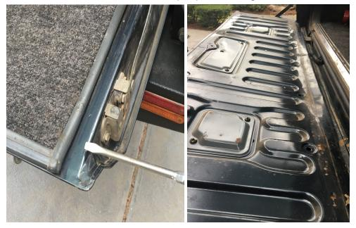
**2.** Remove the three little cover plates that are screwed down, then remove all the small blocks of foam from inside the gate.
