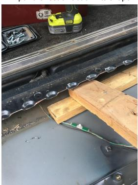
7. Now clean up all the sharp edges with a grinding wheel or file. Then Paint the cut edges so it won't rust.
