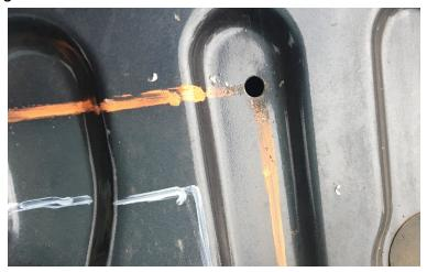
Start cutting in one corner along the line working you way around the hole tailgate, leave some small parts uncut as you go, if you cut the whole thing out in one go, it will flex and vibrate as the longer the cut gets. Once your done go back and cut out those small sections.
