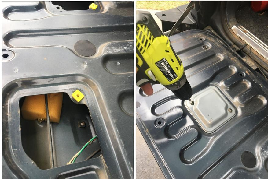
3. Lay out the supplied template, place the bolts into the bolt holes to hold the template down and trace around the inside with a marker or paint pen, then remove it. Before beginning the cut job, we advise covering up the back of your wagon to prevent sharp metal shards from getting it.
