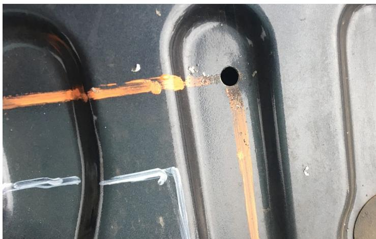
Start cutting in one corner along the line working your way around the hole tailgate, leave some small parts uncut as you go, if you cut the whole thing out in one go, it will flex and vibrate as the longer the cut gets. Once you're done go back and cut out those small sections.
