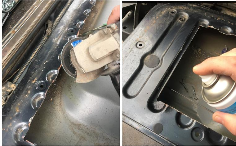
8. Next clean up the inside of the tailgate removing all the metal filing and cleaning the inside with some sort of prep-wash.
