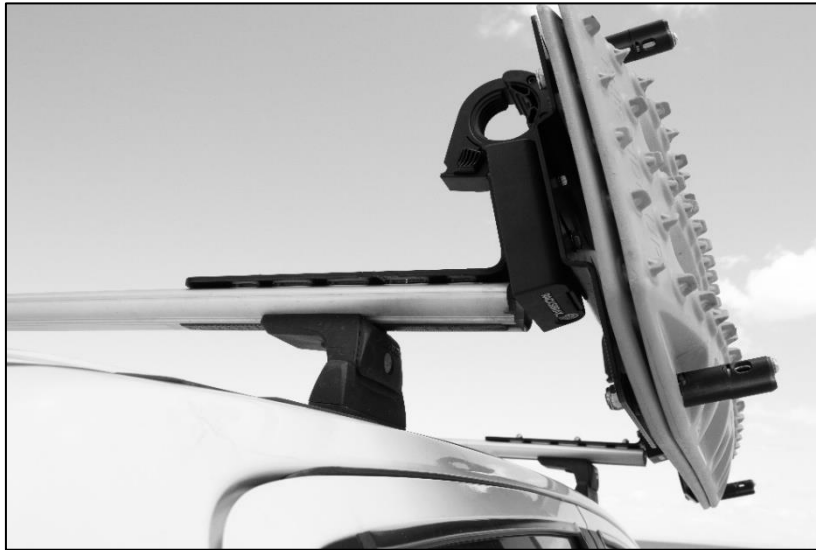
Figure 9 MAXTRAX® side mounted at 15 degrees on roof rack bars
