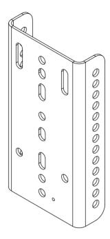
Figure 2 HD/XD Upright Mounting Angle Left (Left) and Right (Right) – Long Slots Uppermost
