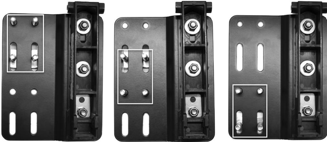
Figure 10 XD Destination Adaptor (Forward) showing the "Washer Frame" at 3 possible heights (High, Middle, Low from left to right) determined by the equivalent height adopted at the Rear Adaptor-view from vehicle side
