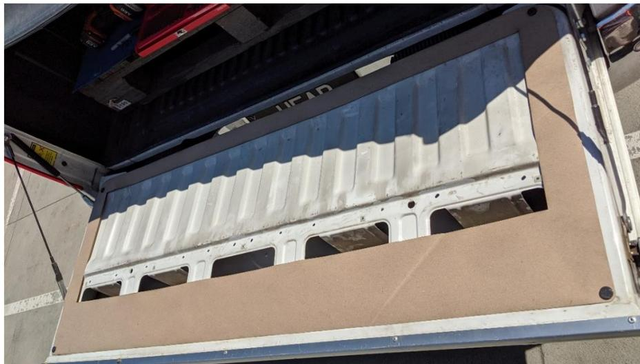
Ensure the template is first centered left to right across the tailgate and parallel to the top of the tailgate. Next adjust the template down so that the internal box will not foul the locking mechanism seen in the image below. Once the template is correctly located, secure it to the tailgate with magnets or weights and trace the perimeter with a marker to indicate your cut path.
