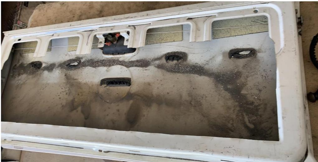
6. Run a bead of Sikaflex® 252 polyurethane adhesive around the perimeter of your tailgate where the provided storage box will rest on your tailgate. We strongly recommend reading the application instructions available on Sikaflex®'s website for full instructions, precautions and cleanup procedure. Most critical though is that you install the tailgate storage unit within ~30 minutes of applying Sikaflex® 252 as once a skin forms on the polyurethane it loses most of its
