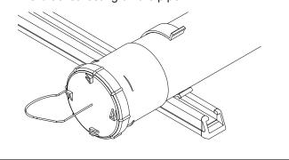
3 Slide the upper C bracket onto the K bracket.
