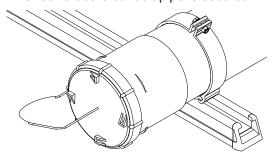
Cut Rubber to fit and install.
