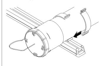
Holding the upper C bracket against the pipe insert the hex bolt, flat washers and nyloc nut. Do not fully tighten the nut. Adjust the conduit pipe to suit the multi slide layout. Tighten the clamp bolt to 10-12 Nm. Check that the conduit pipe is secured.
