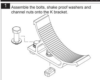
Heavy Duty Bar: Position the K bracket to suit the conduit pipe being used. Tighten the bolts to 10-12 Nm. Channel nuts must be fully located across the cross bar after tightening.
