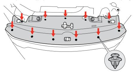
Remove the 11 clips from the upper plastic shroud. To do this, unscrew the centre before pulling upwards.
