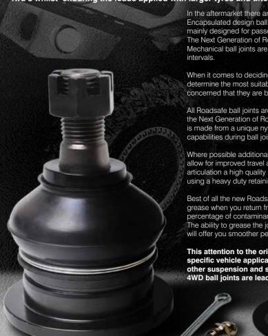
In the aftermarket there are two main types of ball joint – Encapsulated and Mechanical. Encapsulated design ball joints are 'sealed for life' and completely maintenance free. They are mainly designed for passenger vehicles, and offer very little advantage for 4WD applications. The Next Generation of Roadsafe HD 4WD Ball Joints are manufactured in the 'mechanical style'. Mechanical ball joints are not sealed and are supplied with grease nipples for lubrication at regular intervals.
