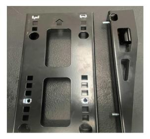
Install spacer onto vehicle using the factory 14mm bolts. Ensure you push the spacer to the centre of the vehicle for max clearance to tail lights for the larger tyres. Make sure the arrow on the spacer is pointing up & place all bolts in loosely before tightening.
