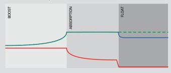
Storage mode - designed to keep your auxiliary battery charged whilst your caravan/camper is in storage by using an eight stage\* charging profile.
