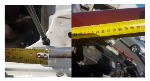
3. Put the strut on bottom ball and bring it up with bracket and mark where to mount. There is enough stroke on the strut to allow the bonnet to lift higher by approx. 100mm. Use a stick etc to hold bonnet higher if you wish, then mark it. You may have to trim back the sound insulation. Mount brackets with nutserts as shown. Keep the strut as square as possible.
