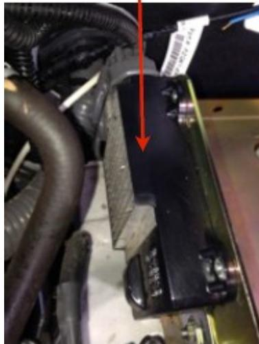
3. Sit battery tray into position. The long support leg towards the firewall of the vehicle requires a 6mm nut and washer that you place on from underneath, and tighten..
