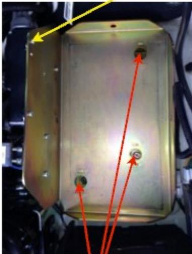
4. Align tray with three existing threaded holes in the skirt, place 3 x 4mm bolts in place and tighten.
