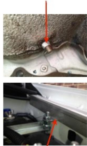
5. Place J hooks in the holes in tray, lower battery in & place hold down bracket on & tighten down until battery is firm. Place a non nylux nut on the J hook on the guard side. Remove 2 x guard bolts, fit support bracket in position. The bracket fits over the J, then place 1 x 4mm nut on & tighten.
