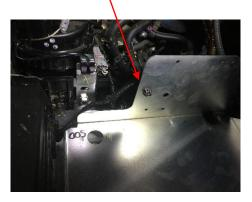
5. Unclip accessories fuse box to fit battery and replace when battery is installed
