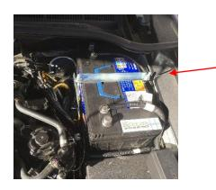
6. Place J hooks in the holes in tray, lower battery in and place hold down bracket on and tighten down until the battery is firm.
