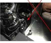
4. Remove clip on sedimenter wire and refit to tray
