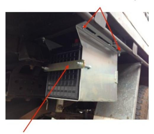
3. Sit battery into box and place battery hold down on, then tighten until battery is firmly in place.
