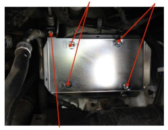
2. There is a black bracket that holds the air con pipe in position. Undo this bracket and remove. Sit battery tray into position, re-use bolt & nut from air con bracket to fix con pipe to the tray. **Make sure you DON'T undo the bolt that joins the air con pipe together, as it will release the air con gas.**
