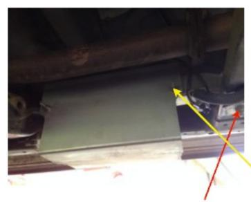
2. Sit battery tray into position. The support leg faces towards the rear of the vehicle. Align the hole in the support leg with hole in the Crossmember. Place 1 x 6mm bolt, washer & nut through hole & tighten.
