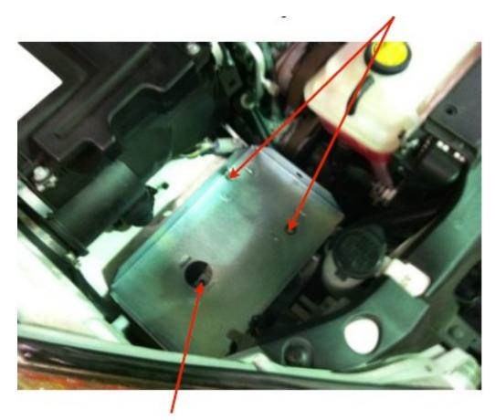
2. Sit battery tray into position. The support leg to the left of the vehicle requires a 6mm bolt & washer.
