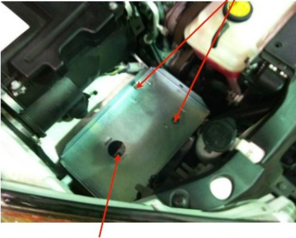
2. Sit battery tray into position. The support leg to the left of the vehicle requires a 6mm bolt & washer.
