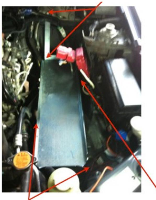
2. Once you remove existing battery tray, sit new tray into place. There is a support bracket to the engine side on the underneath of the tray and one to right front corner, it has an earth wire to it, place 2 x 4mm bolts in these threaded holes.
