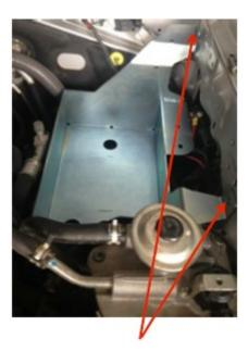
2. There is a module fixed to the skirt in the area where the tray fits, remove and move towards the firewall, re-fix.
