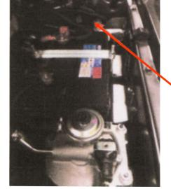
5. Mount BC-DC Unit to batter tray BEFORE installing battery tray per instructions on Page 1.
