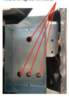
4. Sit battery in tray, fit battery hold down & tighten.
