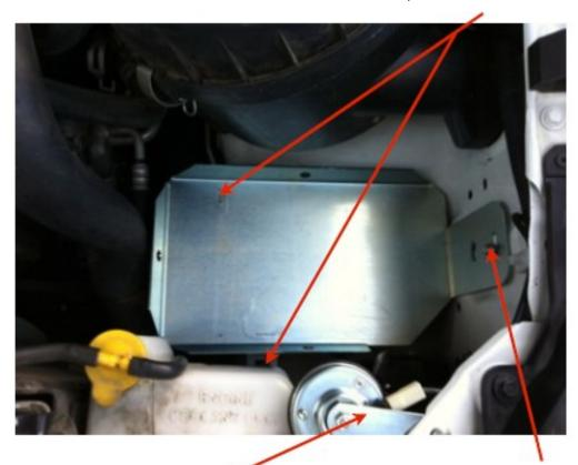
2. Relocate vehicle horn from the skirt to the top locking panel next to the coolant bottle.
