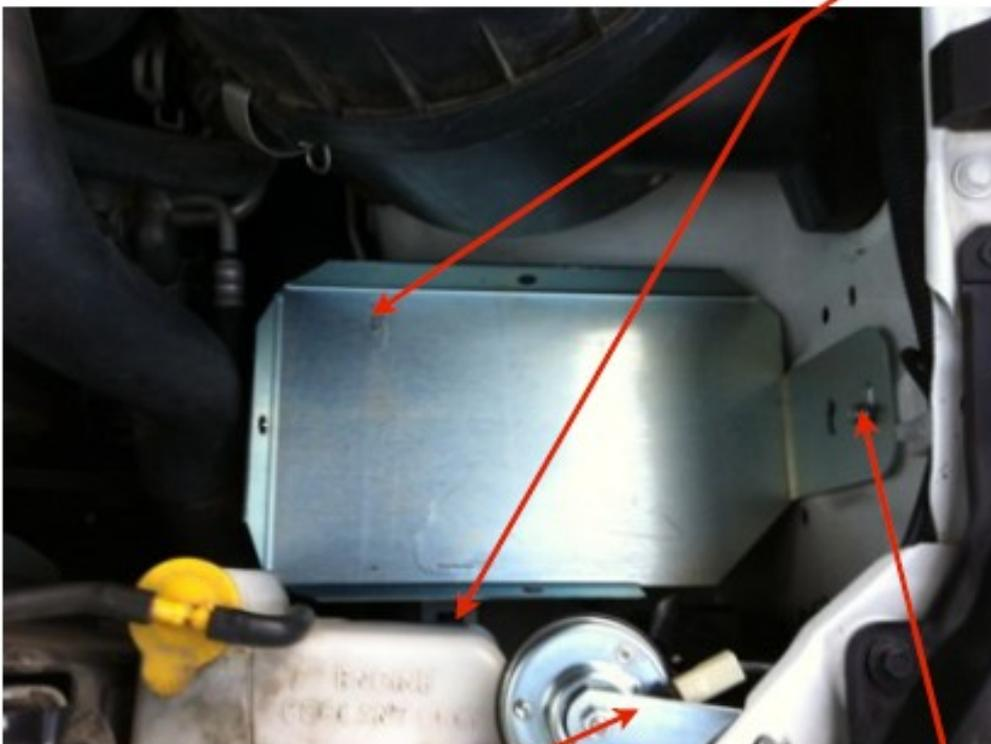
2. Relocate vehicle horn from the skirt to the top locking panel next to the coolant bottle.
