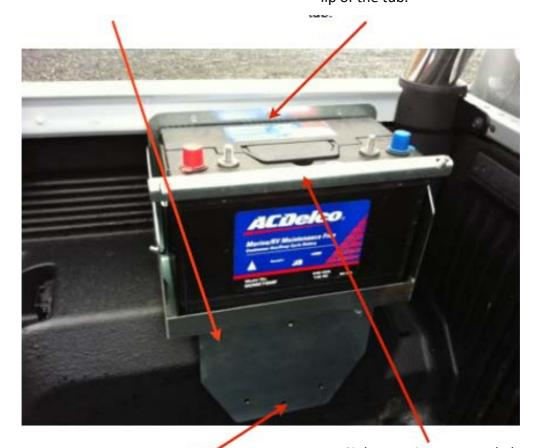
2. Mark holes and drill being careful not to drill into the tyre. Then tighten 3 x 6mm bolts & washers into place.
