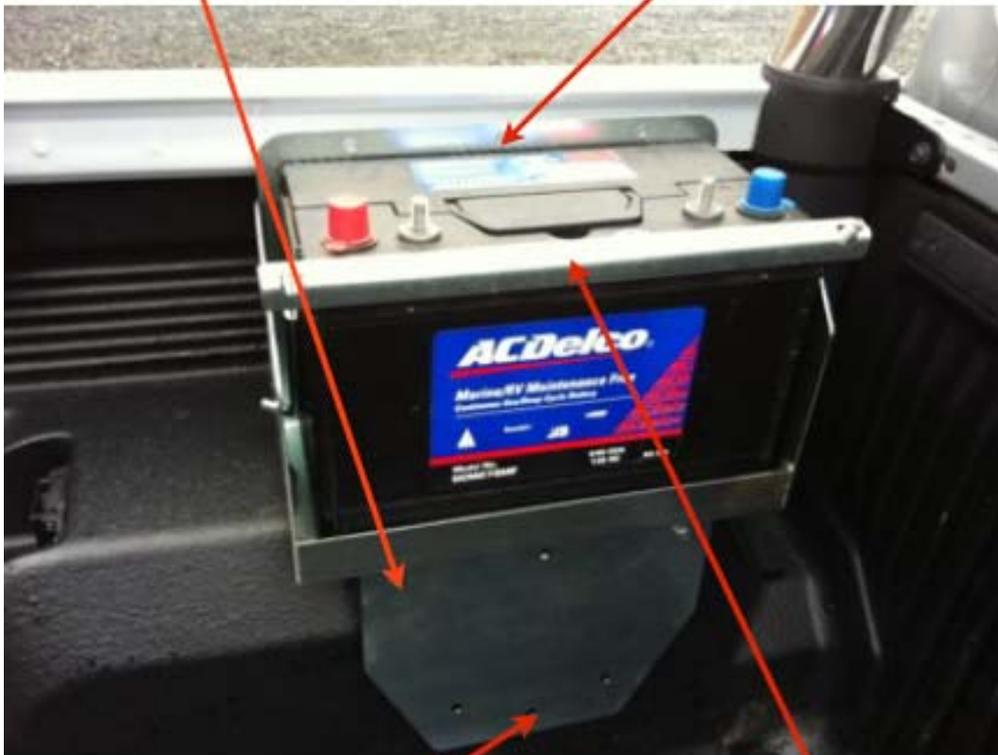
2. Mark holes and drill being careful not to drill into the tyre. Then tighten 3 x 6mm bolts & washers into place.
