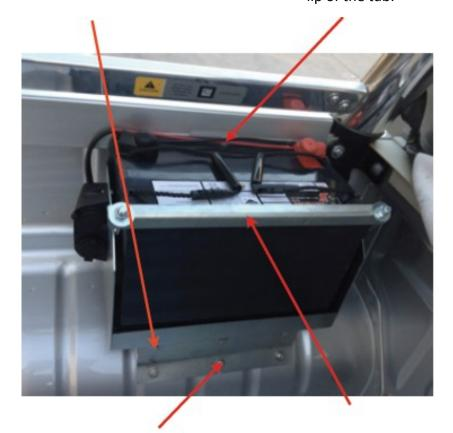
2. Mark holes and drill being careful not to drill into the tyre. Then tighten 3 x 6mm bolts into place.
