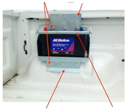
2. Mark holes and drill being careful not to drill into the tyre. Then tighten 3 x 6mm bolts & washers into place.
