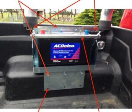
2. Mark holes and drill being careful not to drill into the tyre. Because the tub liner is not hard against the inner wheel arch you need to hole saw 20mm holes in the tub liner & use 10mm thick spacers between the plate and inner wheel arch and then tighten 3 x 6mm bolts, washers & nuts into place.
