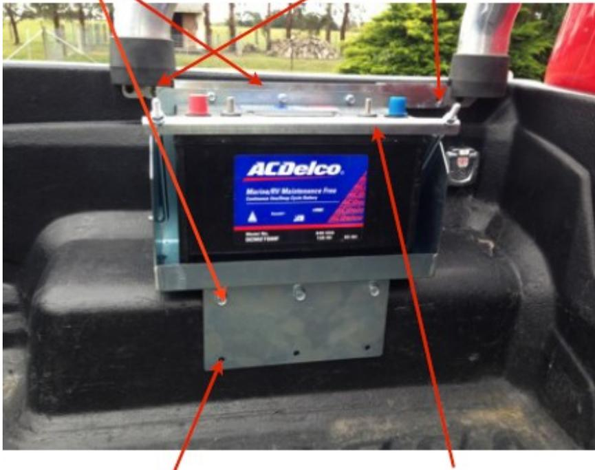
2. Mark holes and drill being careful not to drill into the tyre. Because the tub liner is not hard against the inner wheel arch you need to hole saw 20mm holes in the tub liner & use 10mm thick spacers between the plate and inner wheel arch and then tighten 3 x 6mm bolts, washers & nuts into place.
