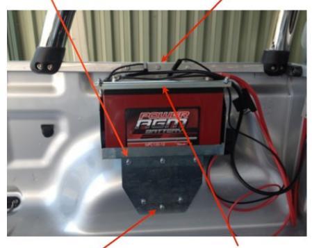
2. Mark holes and drill being careful not to drill into the tyre, and then tighten 3 x 6mm bolts, nuts & washers into place. 4. Sit battery into tray and place battery hold down on the top inner corner of the battery. Put J hooks into the corner holes in the battery tray and through the hold down, then tighten until battery is firmly in place.
