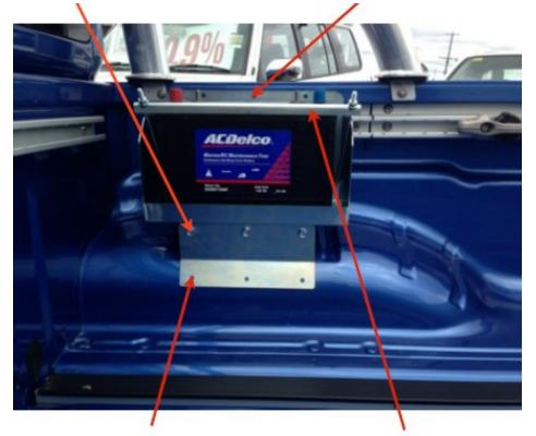
2. Mark holes and drill being careful not to drill into the tyre, and then tighten 3 x 6mm bolts, nuts & washers into place.
