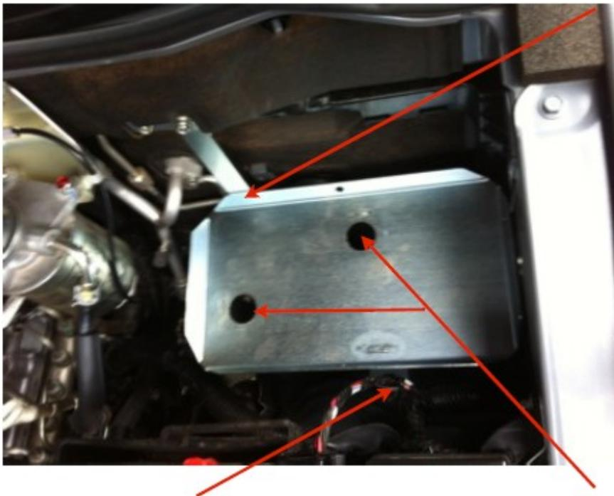
2. Sit battery tray into position. The support leg to the front of the vehicle requires a 4mm bolt.
