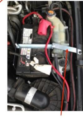
2. Sit battery tray into position. The tray has a support leg under the tray towards the engine and four more mounting points. Fit all 5 x 4mm bolts & tighten.
