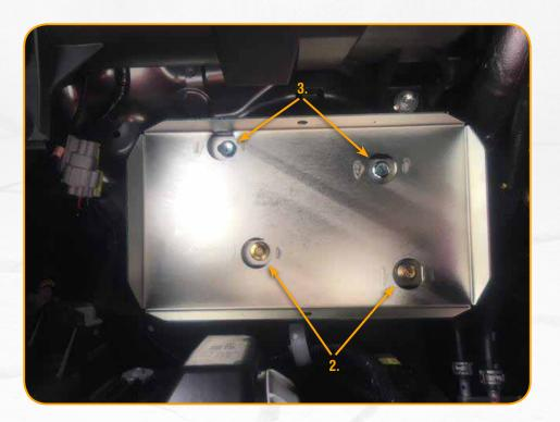
**3.** Then place the 2 x 8mm bolts in the holes at the rear of the tray, use 2 x 8mm nylocks behind the inner guard.
