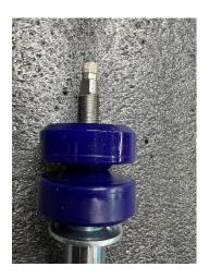
Due to the heavy-duty design of the damper, it may be required to turn the adjusters one or two more clicks anticlockwise in compression and rebound for the first couple of thousand km, to reduce the stiffness and account for a running in period. Please make is full adjustment range on clickers before install as they may be stiff from assembly.
