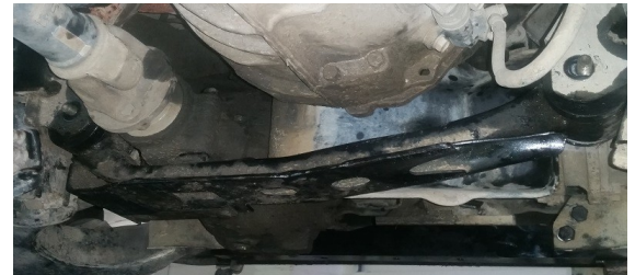
Rear view of rear X member being reinstalled with offset bushings installed.
