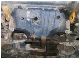
Front factory bash plate to be removed—keep for refitting.
