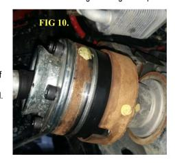
Once all components have been installed in the prescribed order, tighten all bolts to recommended torque values, re-install the bash plates. Now you have lowered the front diff mount, the bash plates will require spacing. Spacers for Bash Plate relocation are not included in the kit.—spacer requirements are specific to Bash Plate brand and design.
