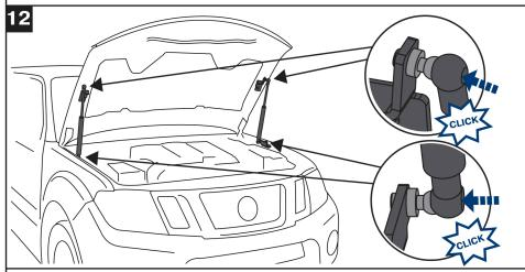
Attention! If it's needed to remove installed gas strut, disassemble how shown on the picture. Operate with the hood being totally open.
