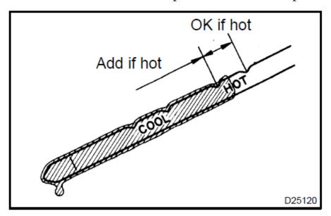
20. To add fluid, insert a clean funnel into the top of the filler tube and slowly pour the fluid down the filler tube. Add small amounts at a time.
