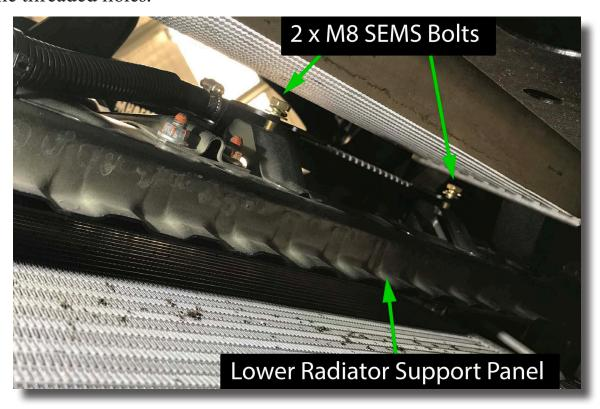
34. Lower the cooler assembly into place while sliding the slotted holes over the M8 bolts in the lower radiator support panel.
