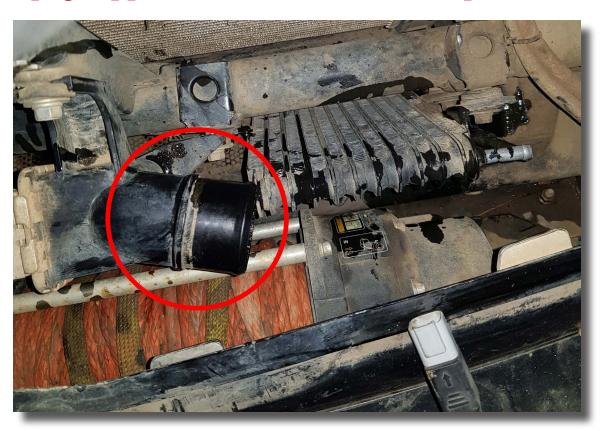
5. Loosen (do not remove) the bolts indicated in the photo below. One bolt attaches the intercooler to the lower radiator support panel. The second bolt attaches the OEM oil cooler to the lower radiator support panel.
