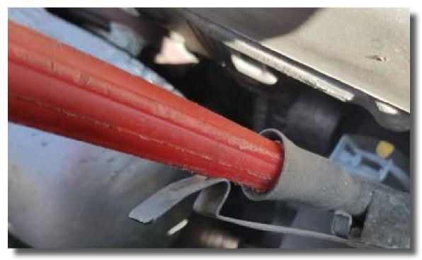
21. Wait 60 seconds before re-inserting the dipstick to avoid false readings from the fluid running down the filler tube.
