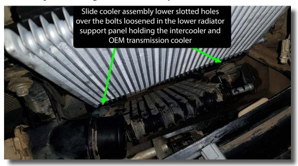
7. Insert one (1) M6 SEMS bolt through the top mounting hole and into the upper radiator support panel and tighten to secure the top of the cooler assembly. Now tighten the two bolts holding the bottom of the cooler assembly to the lower radiator support panel.
