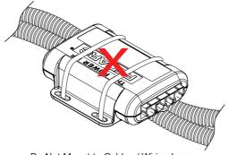
Do Not Mount to Cables / Wiring Looms
