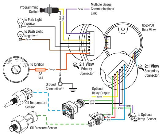
\* Connect to a dash light that dims via the vehicle dimmer adjustment to ensure the gauge dims accordingly. If your illumination circuit in your vehicle varies the positive voltage for dimming you will require an Redarc Enhanced Lighting Controller (GA-ELC) to get the gauge to dim with you night-time driving lights.
