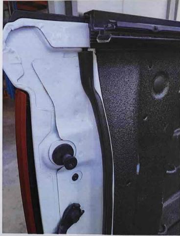
2: Install the two side seals following the body line as pictured. Only peel 100mm of backing at a time to give you control in placing the seal. The adhesive is very strong and will not release withoust tearing the rubber.
