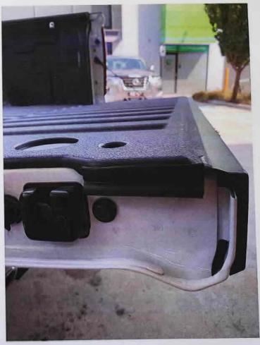
3: Install the pinchwelds by pressing them to the underside lip of the tubliner on each side
