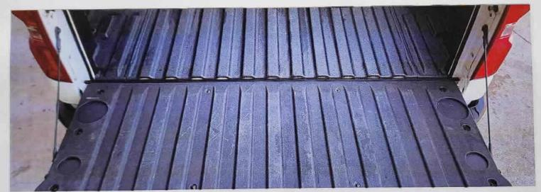
1: Install the long seal to the body keeping it tight to the underside of the tubliner as pictured
