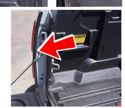
4: A secondary side seal is fitted so it closes against the pinch weld on the tub.
