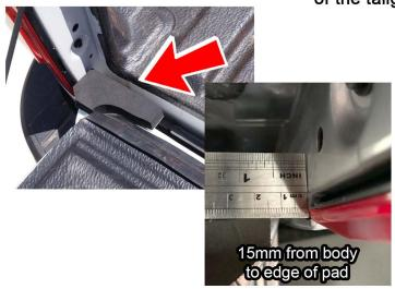
3: The side seals are fitted on the body edge over the tail light as shown. You will need to lift the tailgate slightly to take the tension off the stays so you can pass the seal between them and the body. The seal should be cut so the inner top lip of the gate does not drag over it
