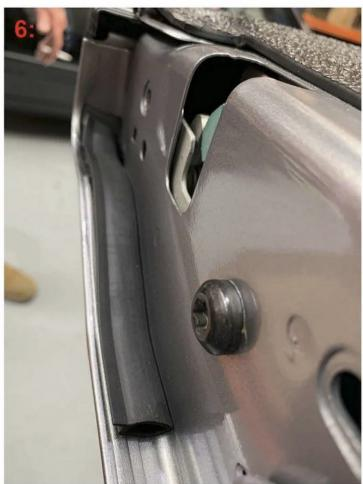
6: Install the 150mm seals to each side of the top of the tailgate as shown above
