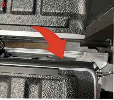
5: Attach the 1305mm long seal the bottom of the tailgate as shown
