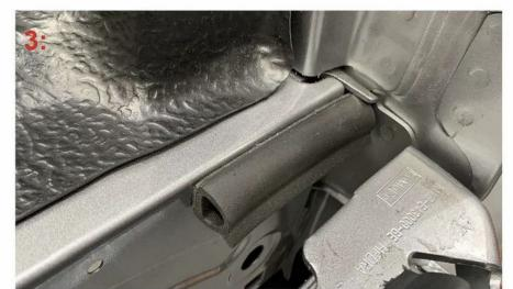
3: In each corner of the tub install the 80mm seal as shown
