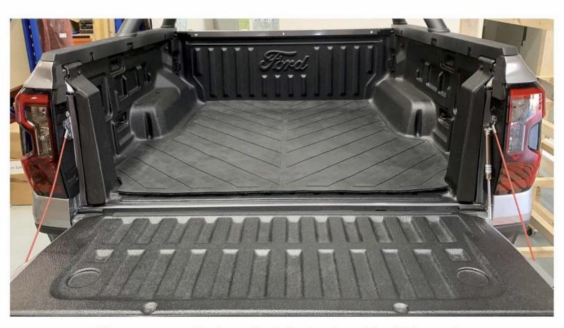
We recommend to keep the tailgate closed for 24 hours to let the seals compress and the glues adhere
