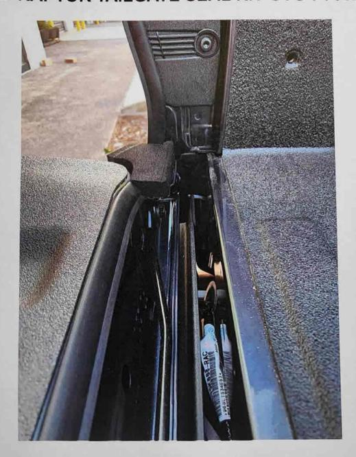
4: Following the edge of the tailgate install the long seal as pictured. If you find you have to much length once you finish simply trim it to fit tight between both foam pads.
