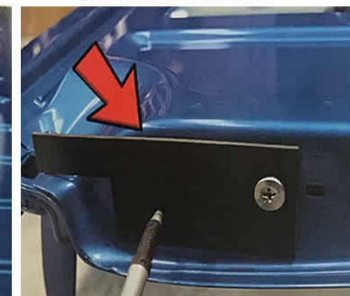
Bolt on the template as shown & mark the tailgate as shown
