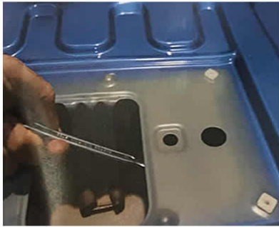
Hold the friction nut inside the tailgate with a 12mm spanner
