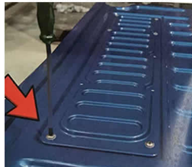
Remove tailgate access panel bolts as shown
