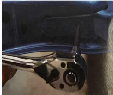
Remove the tailgate hinge bolt closest to the body
