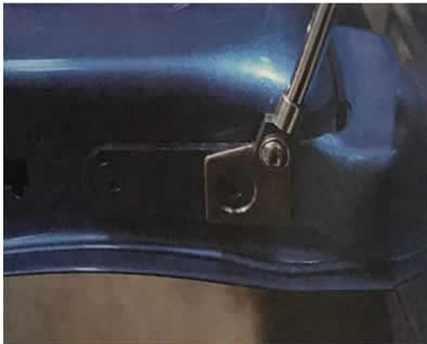
Install the strut as shown the replace & tighten the bolt
