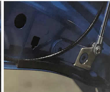
Install the cable locating rubber 80mm back from the body as pictured
