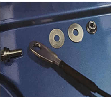
Installing the cable to tailgate
