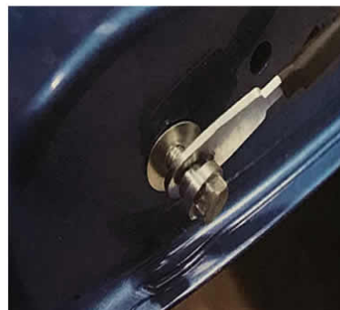
Place bolt supplied through the hole placing thin washer against tailgate first
