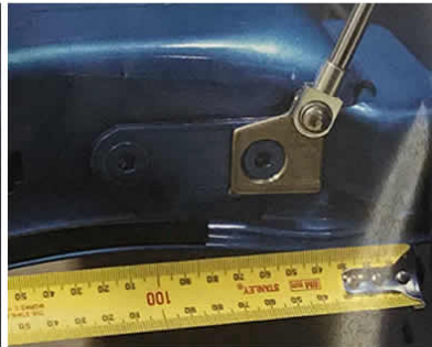
Install the cable locating rubber 80mm back from the body as pictured
