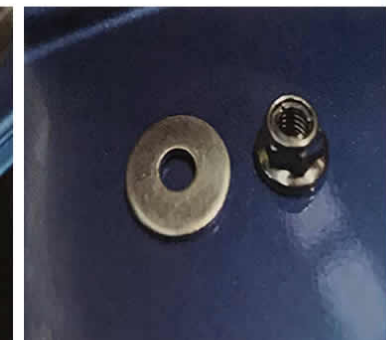
Screw the friction nut inside tailgate placing thicker washer on first
