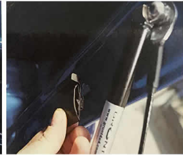
Remove the rubber locating blocks from the tailgate & ute tub
