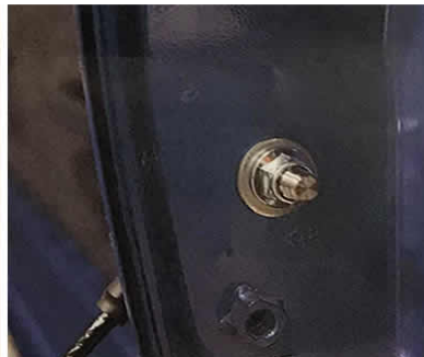
Place the thicker washer on the back followed by the friction nut then tighten
