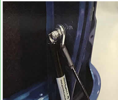
Insert the strut & strap through the holes as shown placing the thin washer against the body
