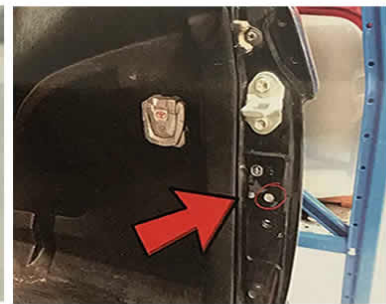
Factory hole that the Down Strut Mounts to
