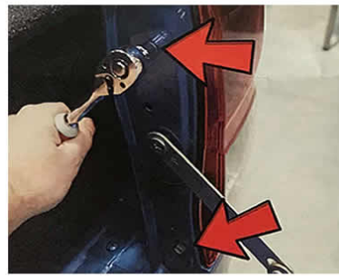
Remove the two Tail light Bolts followed by the light assembly
