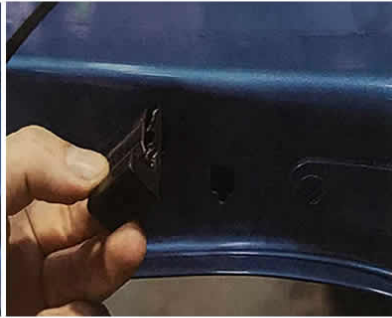
Remove the rubber locating blocks from the tailgate & ute tub
