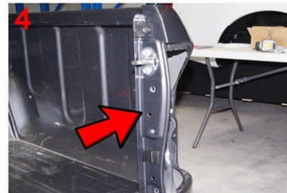
4: Factory hole that the DOWN strut mounts to
