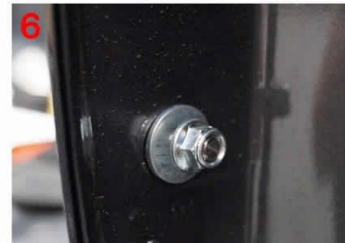
6: Place the thicker washer on the back followed by the friction nut then tighten
