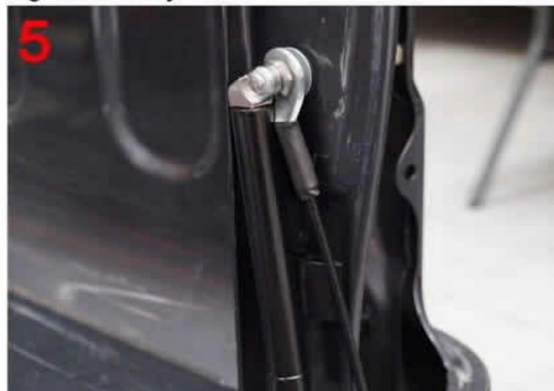
5: Insert the strut & strap through the hole as shown placing the thin washer against the body
