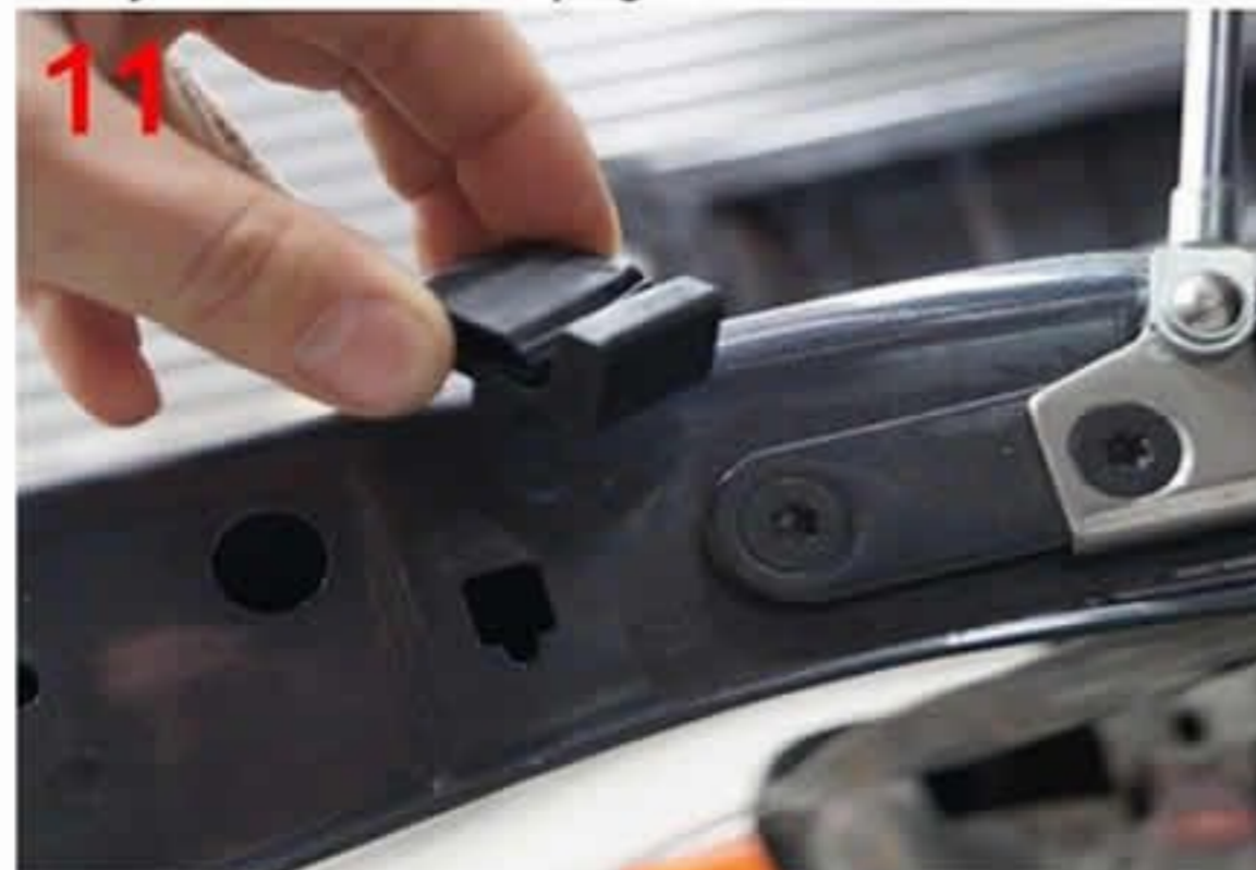
11: Remove the rubber steel strap locator from the tailgate
