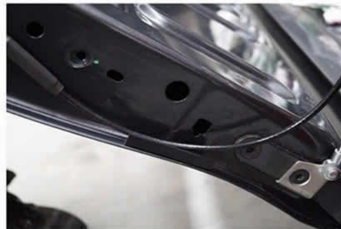
13: Install the cable locating rubber 130mm back from the body as pictured
