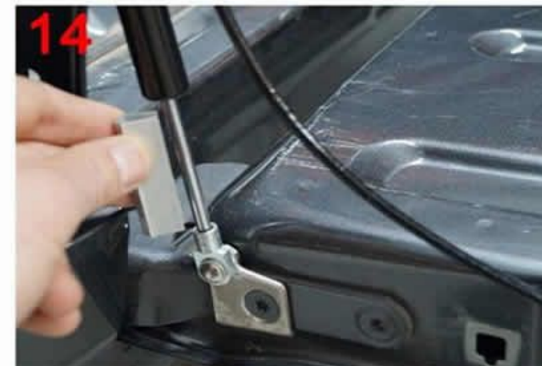
14: Repeat the process on the passenger side for the EASY UP strut removing the spacer once installed
