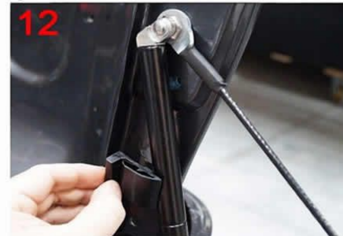
12: Remove the rubber steel strap locator from the body
