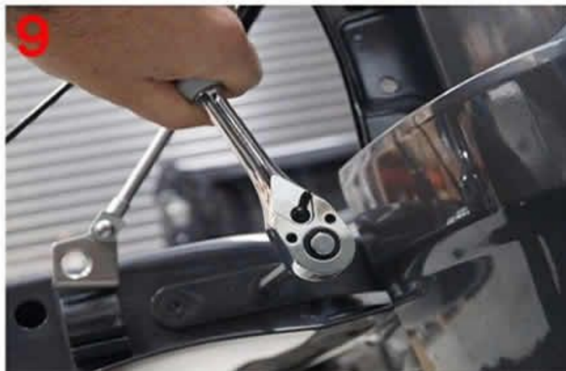
9: Remove the tailgate hinge bolt closest to the body *see notes on page 3
