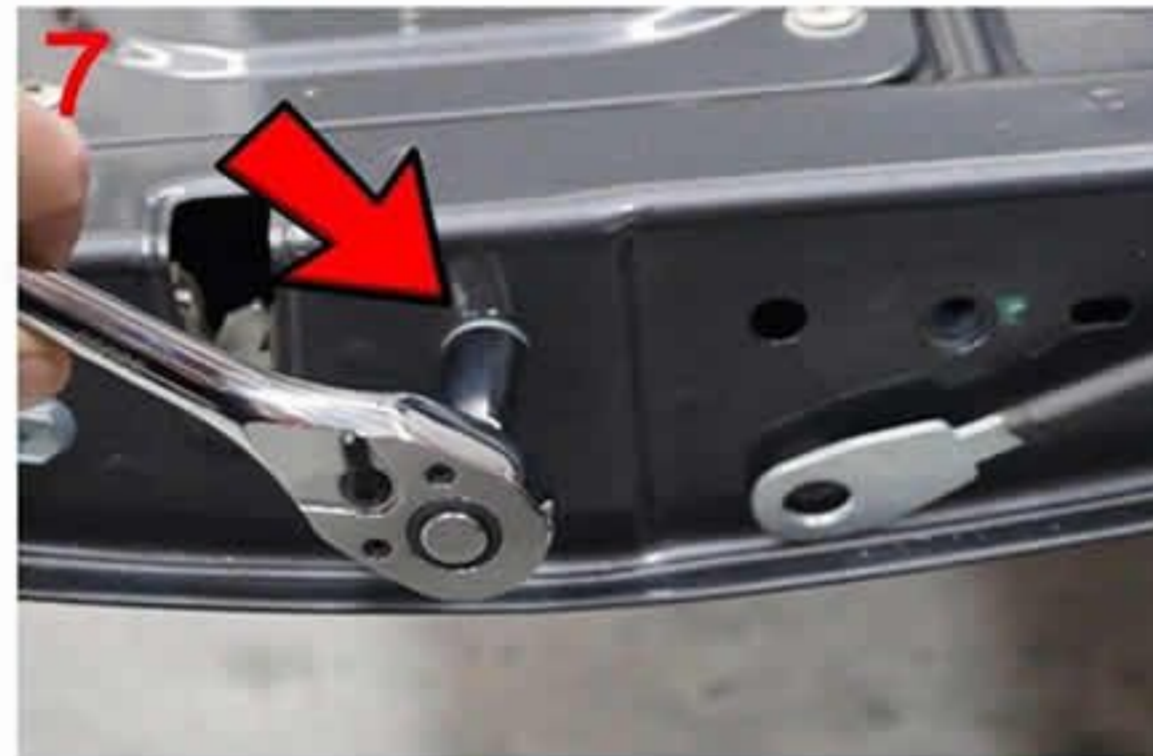
7: Remove factory bolt as shown
