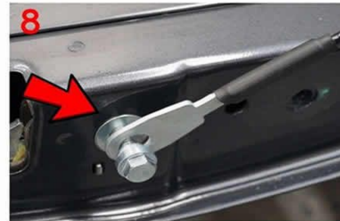
8: Replace with new bolt provided placing thin washer against the tailgate first
