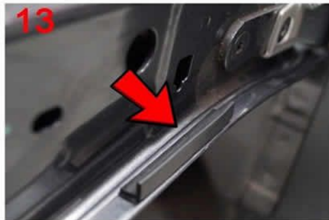
13: Install the cable locating rubber 130mm back from the body as pictured
