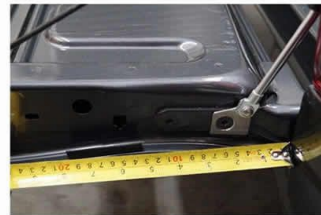
13: Install the cable locating rubber 130mm back from the body as pictured
