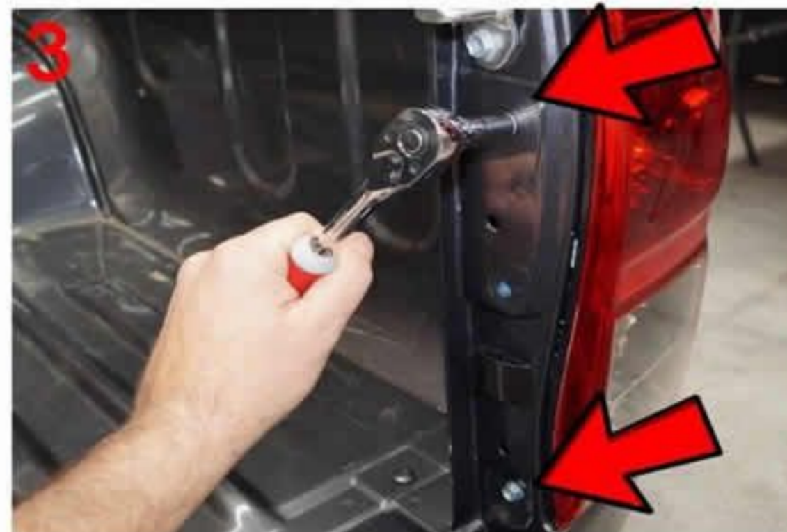
3: Remove the two tail light bolts followed by the light assembly
