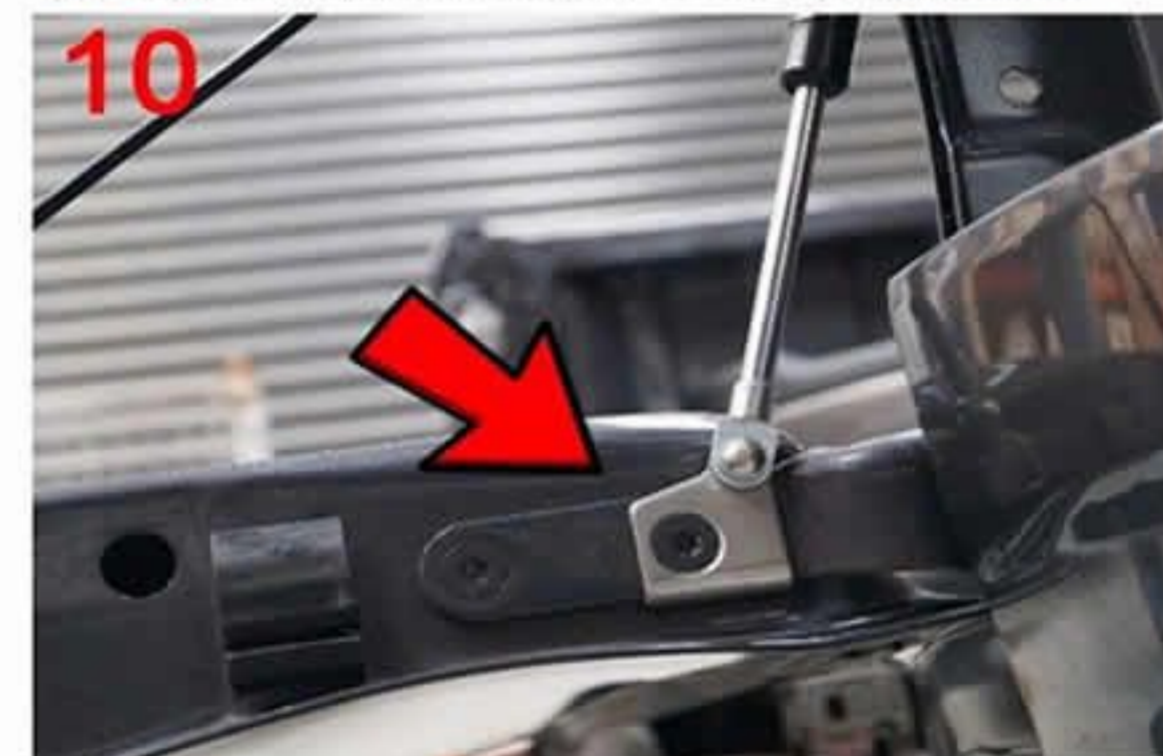
10: Install the strut as shown then replace and tighten the bolt
