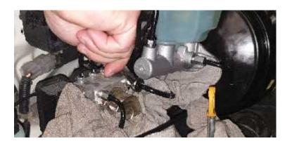
Now remove any air caught in the pipe between the master cylinder and ABS pump. Using a pipe spanner, loosen the **fitting on the ABS pump** while another person gently applies the brake pedal. Brake fluid and any air should come out of the fitting. Tighten the fitting before brake pedal is released.
