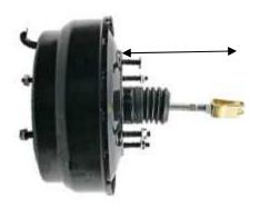
On the original booster, measure the distance from the fire wall face to the pedal mount and adjust the new booster to the same length.
